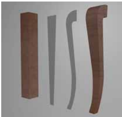
Figure 3: Leg templates are created in form•Z to create the rough leg form.
