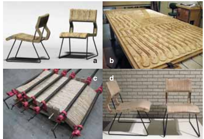
Figures 13: Furniture Design: “Wally’s Chair” by Nate Moren. (a) form•Z rendering of the chair model. (b) OSB panel on the CNC router after cutting the sections for one chair. (c) Stack lamination: OSB components assembled on the laminating jig. (d) Two of the finished chairs.
