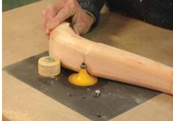
Figure 6: 'Controlled rounding' conducted using the router table.
