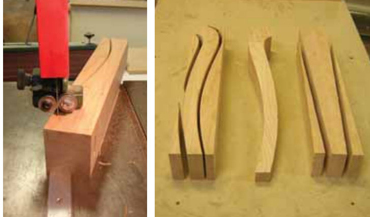
Figures 4,5: 'Boolean Operations' conducted using the band saw tool in the workshop.
